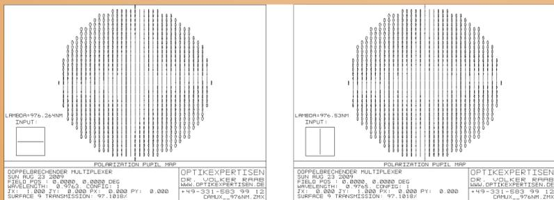
A simulation of the filter characteristic of a 10mm long calcite crystal is shown. On the left light of 976.264nm with horizontal polarization is incident; on the right 976.530nm with vertical polarization. Both beams exit with vertical polarization. The degree of rectification is decreasing with increasing divergence. The extension of the plot is about  $\pm 40$ mrad.
