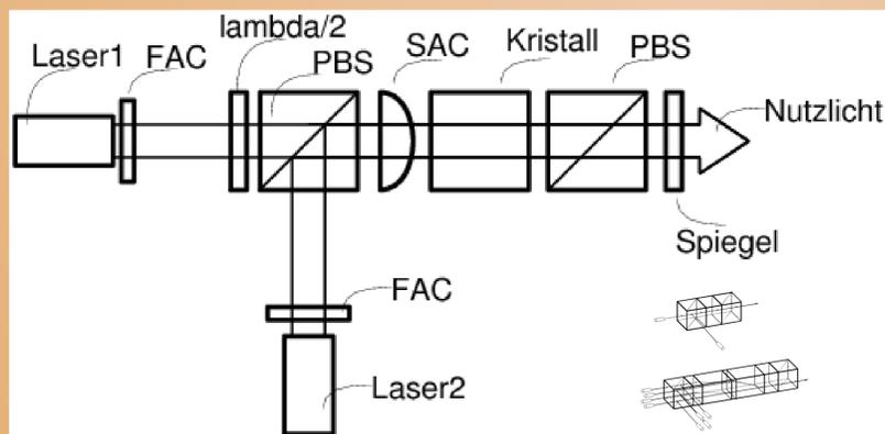
Two (semiconductor) laser are polarization coupled. The combination of a birefringent crystal between two polarizers operates as a narrow bandwidth Lyot-filter. The laser lines lock to their respective wavelengths by means of a feedback-mirror. Due to the polarization beamsplitter the two laser emissions are orthogonal on the side of the semiconductors and parallel on the side of the outcoupling mirror.
