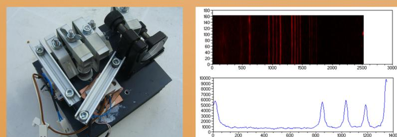
A demonstrator (ca. 10x10cm<sup>2</sup>) with two broad area diodes (150 $\mu$ m width) has been set up.
