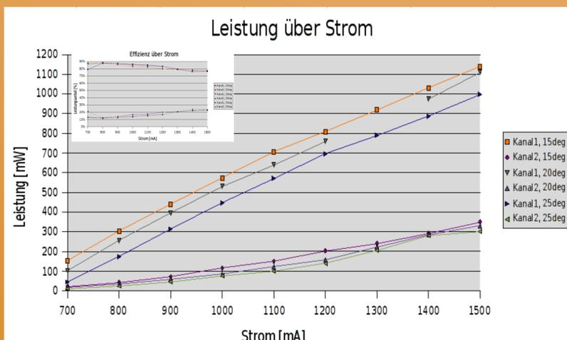
For three different temperatures of the heat sink the combined output power has been determined. It reaches more than 1W for temperatures below 20°C. Also given is the power in the "loss channel" out of the second PBS. The relative powers define the coupling efficiency.
